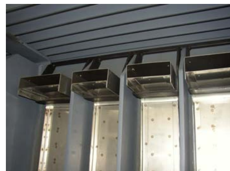
Figure 4. SHEs mounted using a simple one-piece hanger in central inter-cradle space of the demonstration model
