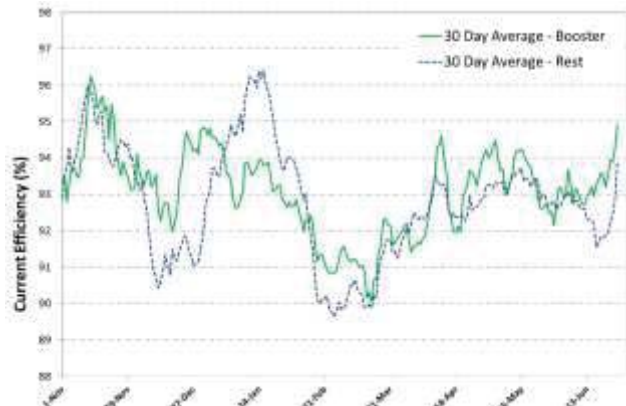
Figure 11 - Trial group current efficiency (%) compared to rest-of-line average over extended trial period
